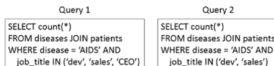
Figure 11: Difference attack using victim in IN clause. This attack is actively detected and prevented.
